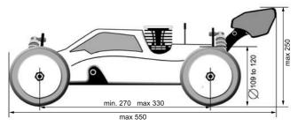
Wheel overall diameter must be between 109 and 120 mm. Wheel overall width 47 mm maximum.
