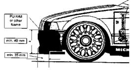
1:1 car construction to absorb impact energy.
